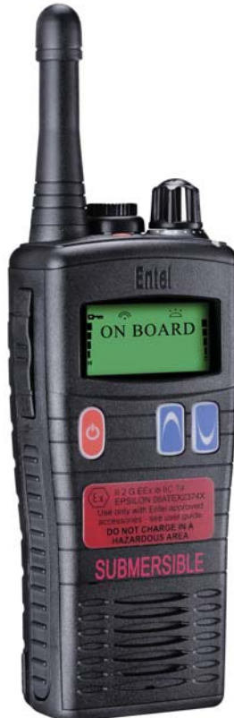
Pictured: UHF ATEX variant with stubby antenna
